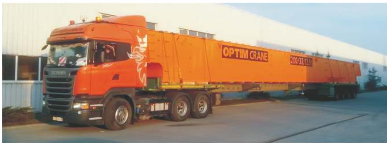
Transporting span beam bridge crane - load capacity 200/32/12,5 t, Verkhny Tagil GRES
