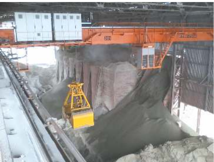
Grab crane – capacity load 20 t, Kazakhstan
