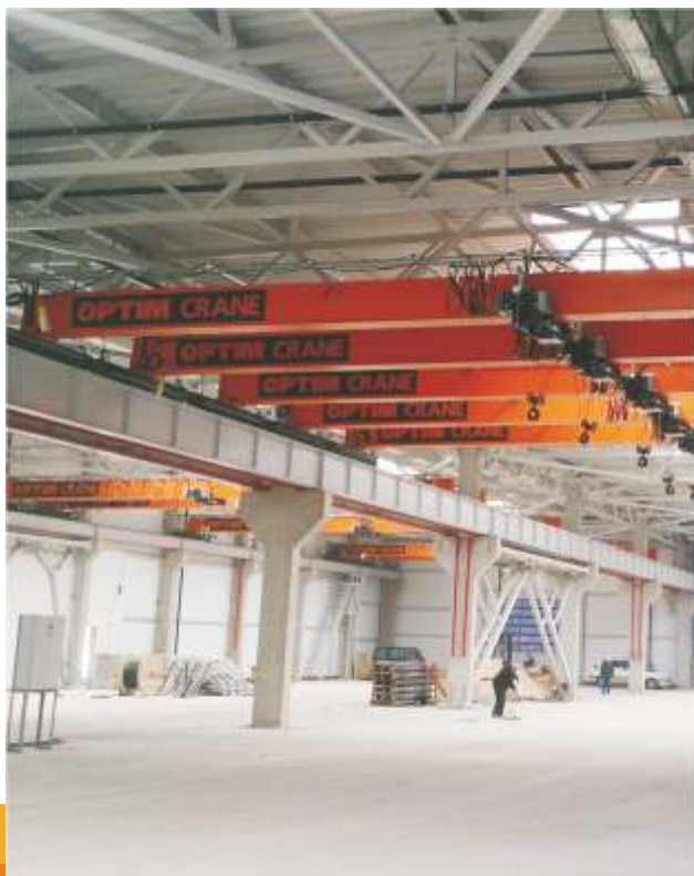
10 pcs of cranes of load capacity 5t, the new fabrication shop. Vnukovo
