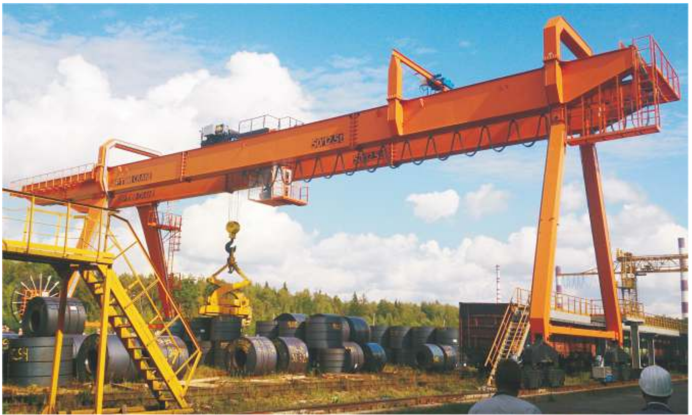
Gantry crane of load capacity 50t, span – 32 m. Gazpromtrubinvest. Volgorechensk.
