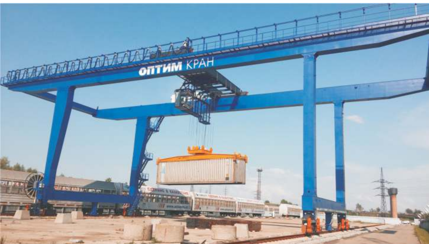
Gantry cranes container for 20 ft, 40 ft container. Asia-Auto, Kazakhstan
