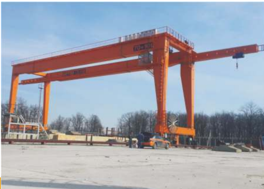
Gantry crane of load capacity 70t, span – 42 m. Stoilensky GOK. Stary Oskol
